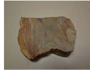
Two photos of each side are shown. Size is about 190mm x 100 mm and 55 mm thick. Near the left are signs of the central pith indicating the diameter was about 380 mm after mineralization. It is hard to estimate the tree age as counting growth rings is difficult.
